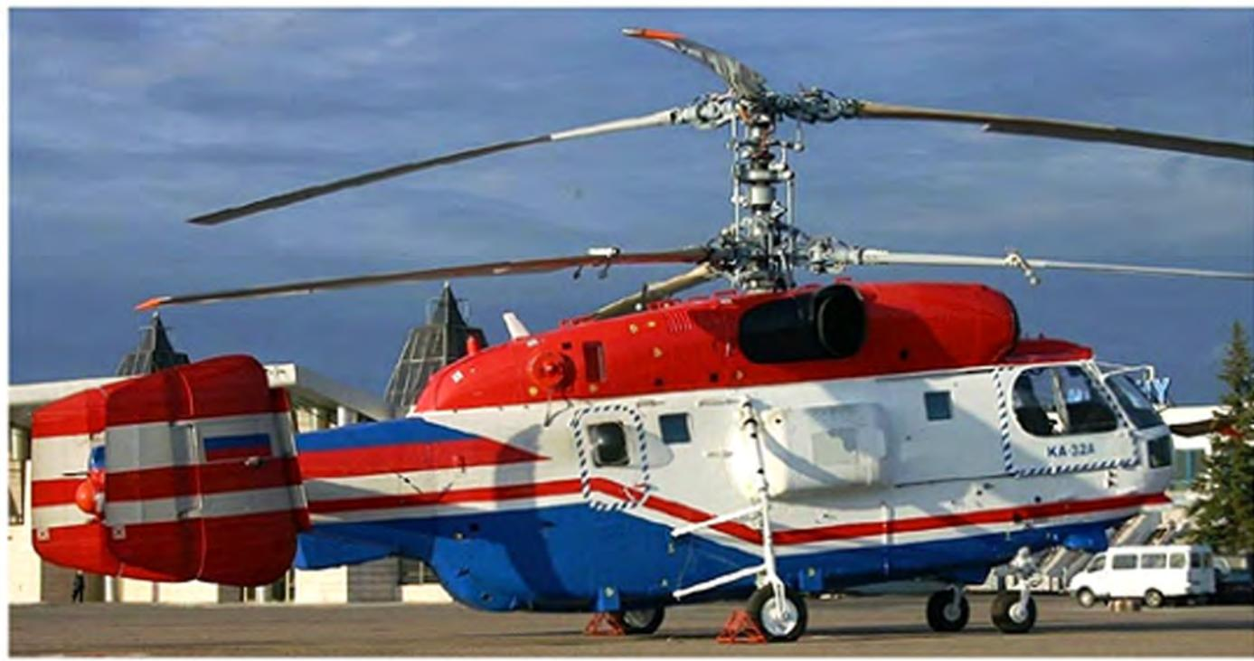
The Kamov Ka-32A is an autonomous high-power-to-weight-ratio compact air transporter that can operate independently of ground support. The main roles of the Ka-32A civil helicopter are as passenger and cargo transport, a flying crane for building construction, transport for bulky cargo up to 5t carried on an external sling, logging, search and rescue, medical and emergency evacuation, loading and unloading ships at sea and offshore operations.
